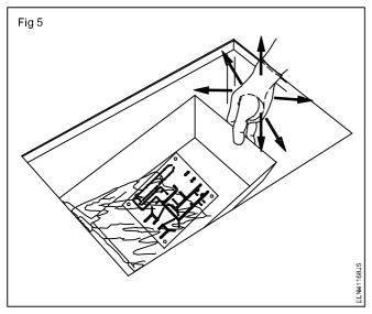
5 Repeat step 4 for 10-15 minutes and observe the unpainted portion of the copper clad getting etched OFF.
