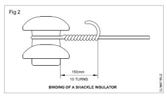
11 Bind the shackle insulators with the one fixed at the last cross - arm.
