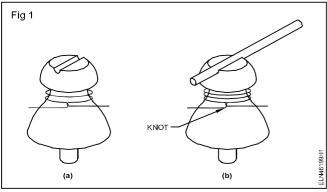
7 Make a knot of the binding wire with the free ends tightly. (Fig 1b)
