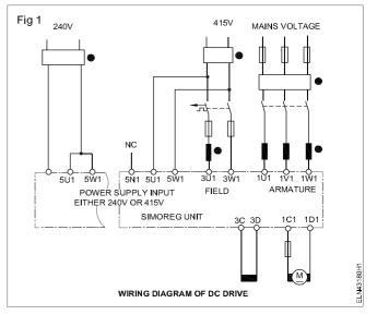
7 Check the supply and ensure for proper rating of fuses main switch according to the motor rating.
