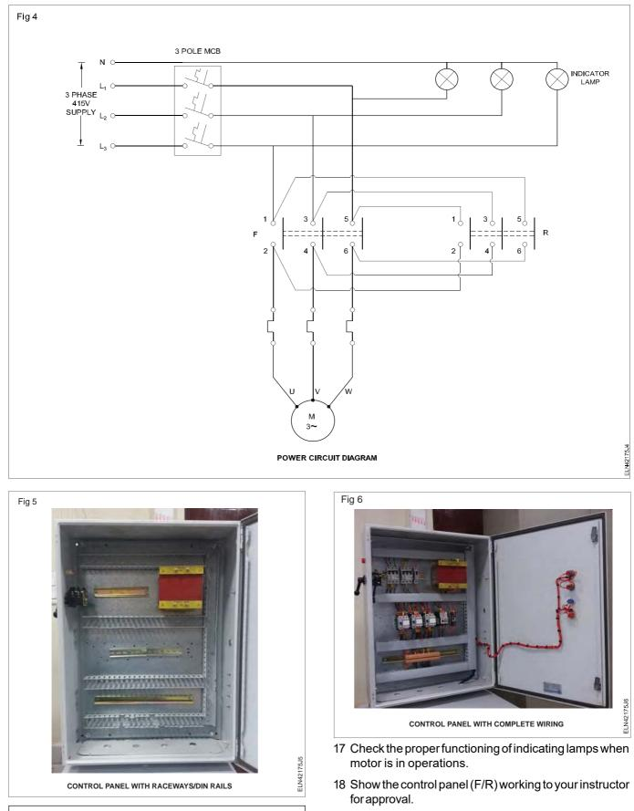
A typical control panel with complete wiring is shown in Fig 6.
