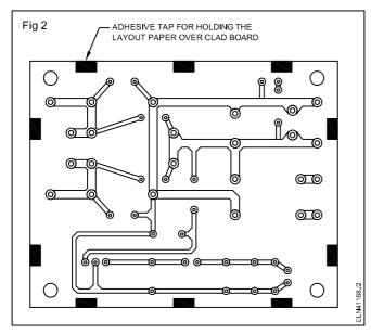
5 Make punch marks using a centre punch, at the centres of all inner circles and the mounting hole circles.
