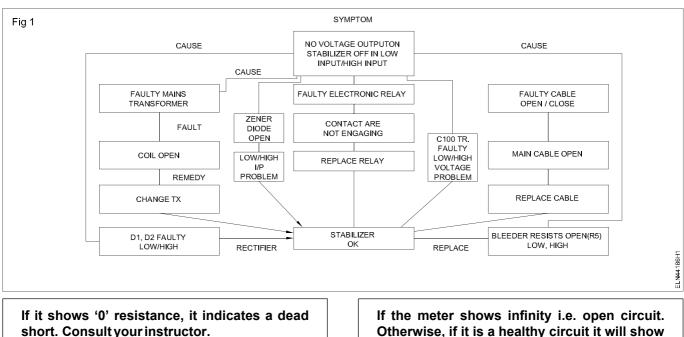
3 Check for any open circuit visually or by ohm meter after testing for short circuit.
