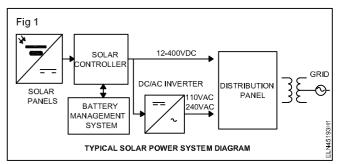
Fig 1 is the model schematic diagram of solar power plant given for the general guidance of trainees. The trainees have to prepare and draw the schematic diagram of the solar power plant they visited.
