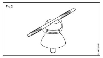
Binding should be tighten without any gap.
