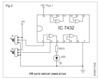
4 Set switches SW<sub>1</sub> and SW<sub>2</sub> to apply input logic levels as in Table 3 to the first OR gate (Fig 2). Record the output logic level and verify its truth Table 3.
