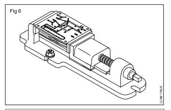
Drill slowly and steadily. Careless drilling may pull the complete circular copper pattern away.
