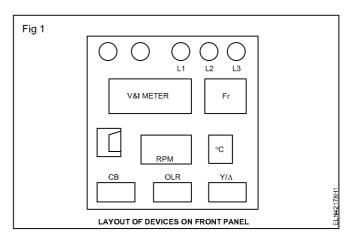
6 Wire the fitting in front panel using suitable cables.
