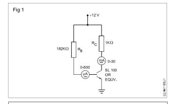
The transistor is heated to observe the effect of heat on the set Q point of the transistor.
