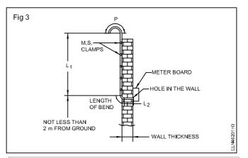
The hole should not be less than two metres from the ground.
