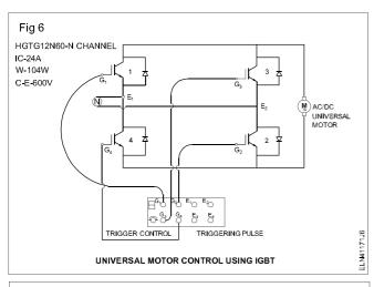
1 Wire the circuit as per the diagram. (Fig 6)
