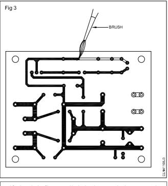
If the ink flows slightly beyond the traced pattern circles and lines, do not try to correct it.
