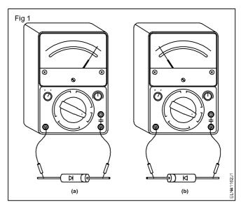
If the meter reads low resistance for both polarities the diode is short.
