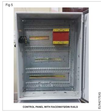
5 Run the wires in the race ways one by one. Avoid the cross over of the wires.
