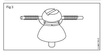
9 Complete the binding by giving about 15 turns on both sides.
