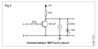
2 Power ON the circuit, by applying 5V Fig 5. Apply logic level-0 to the input (see note below) and record the voltmeter reading, its equivalent logic level and the status of LED.
