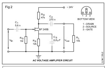
Construct the circuit on a bread board or on a GPCB. If you are wiring the circuit on a GPCB use base for the FET to ensure that it does not get damaged.
