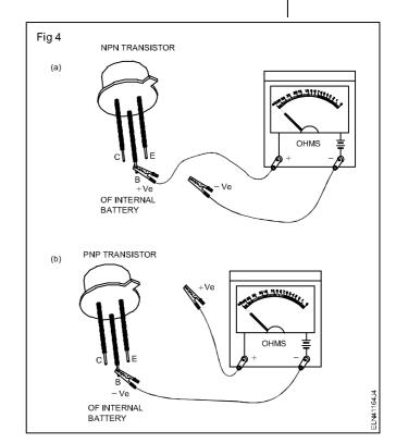
Electrical : Electrician (NSQF LEVEL - 5) - Exercise 4.1.164 Copyright @ NIMI Not to be Republished 5 From the recorded observations in steps 3 and 4, and referring to the table given below, conclude and record, the condition of the base-emitter junction diode of the transistor as GOOD, open or shorted in Table 3.
