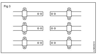
If any over lapping ends of the busbar join by bolting together.
