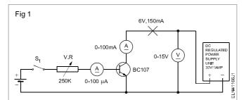
Check for the specific range of instruments and correct polarity.
