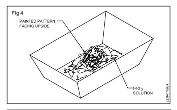
Do not agitate the solution very fast as this may sometimes peel off the paint and etch the required patterns also.
