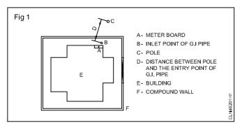
Care should be taken to see that the service cable does not cross the adjacent building area. In some cases an intermediate pipe structure may be needed to avoid crossing.
