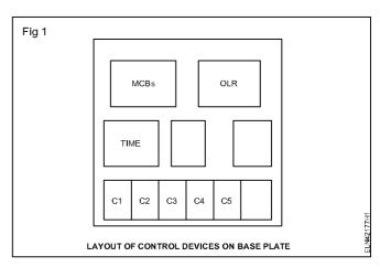
5 Fix the devices according to the layout on base plate check each devices for its rigidity and position correctness and get it checked.
